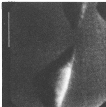
Fig. 2. Oxide nuclei formed at 798 K, SEM \times 30,000 , 15 kV, surface 30^\circ tilted, length of marker 1 \mu\text{m} .
